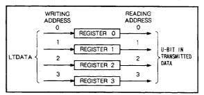
Fig. 3 The structure of U-bit data registers
