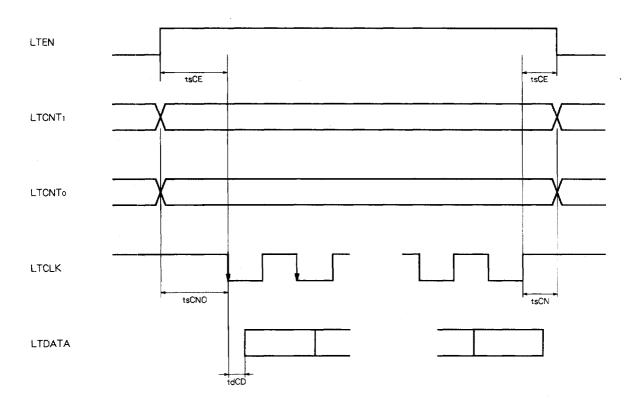
Note: As internal registers for data output are set at edges of the LTEN, LTCNTO, and LTCNT1 signals, at least one of these signals must be inverted in advance to read out status, C-bit data, and U-bit data.
