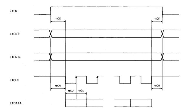
Note: As internal registers for data input are set at edges of the LTCNT0 and LTCNT1 signals, at least one of these signals must be inverted in advance to write settings, C-bit data, and U-bit data.
