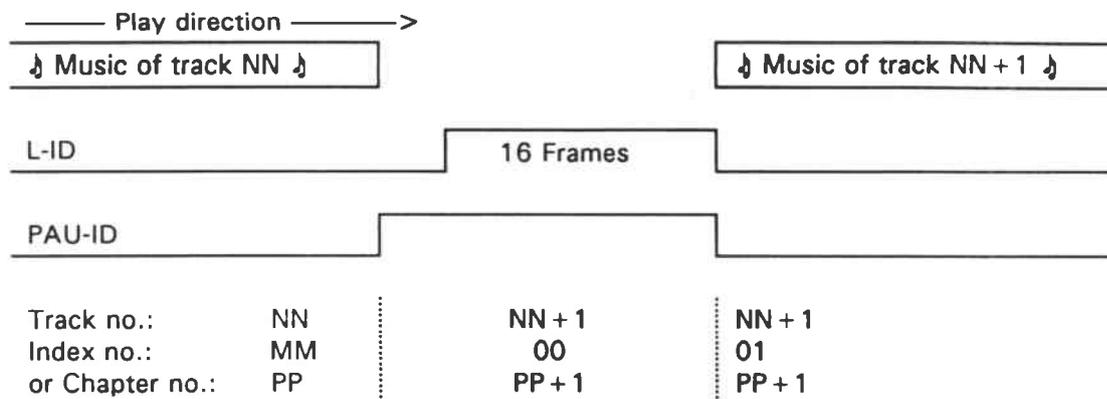
The trailing edge of the L-ID coincides with the trailing edge of the P-ID.
