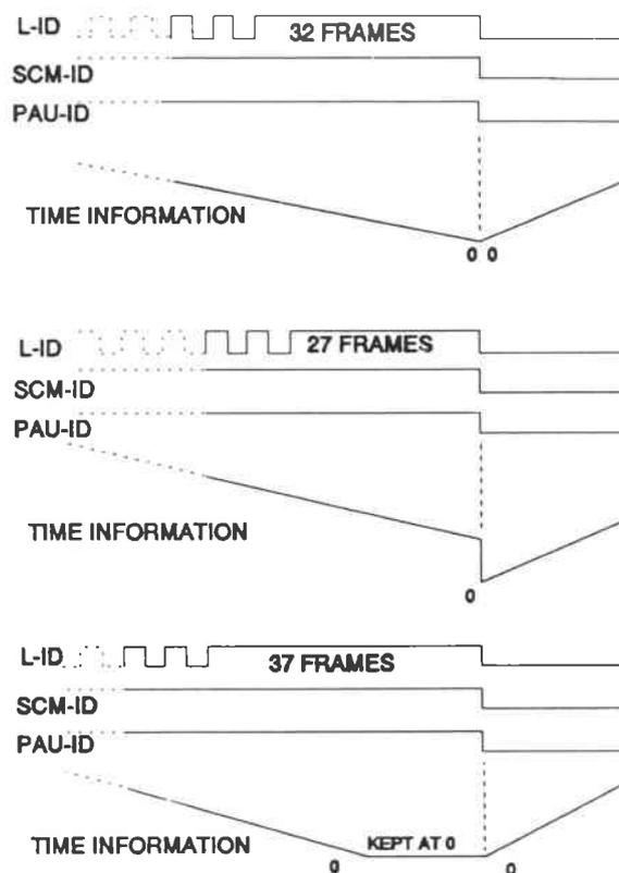
If the last part of the Lead-in (the 32 frames nominal) is longer than 32 frames the absolute time is kept 0 for some frames. If the length is less than 32 the absolute time will not decrease to exactly 0.
