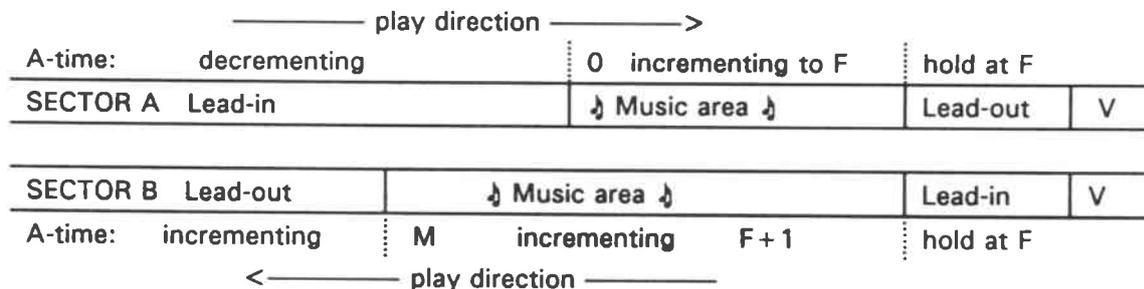
In the Lead-in of Sector A the A-time will decrement to 0:00:00:0 until the final frame of the Lead-in area, with an accuracy of -0/+ 5 frames (the time information may not be negative). It will be recorded in ascending order from there on, until the last frame of the music area, whose A-time is indicated here by "F".
