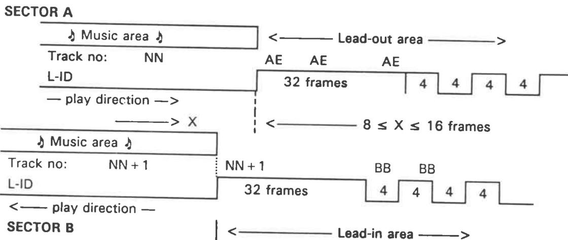
The position of the rising edge of the L-ID at the end of Sector A should be at least 8 frames, and a maximum of 16 frames before the start of the first track on Sector B.
