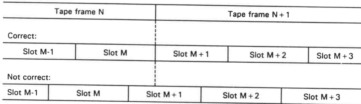
The PASC Slot is converted into a Tape frame slot as shown below:
