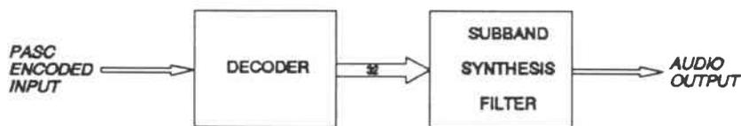
This section contains a description of the decoding according to the PASC system. Two major blocks are the transformation of the PASC bitstream into subband data and the subband synthesis.
