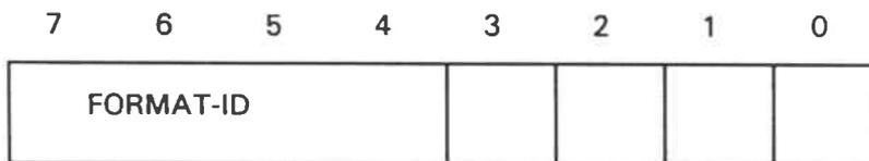
Bits 7-4 of byte  $SI_0$  indicate the application of the Main Data and are referred to as FORMAT-ID. The contents are the same as the FORMAT-ID in the Auxiliary Data:
