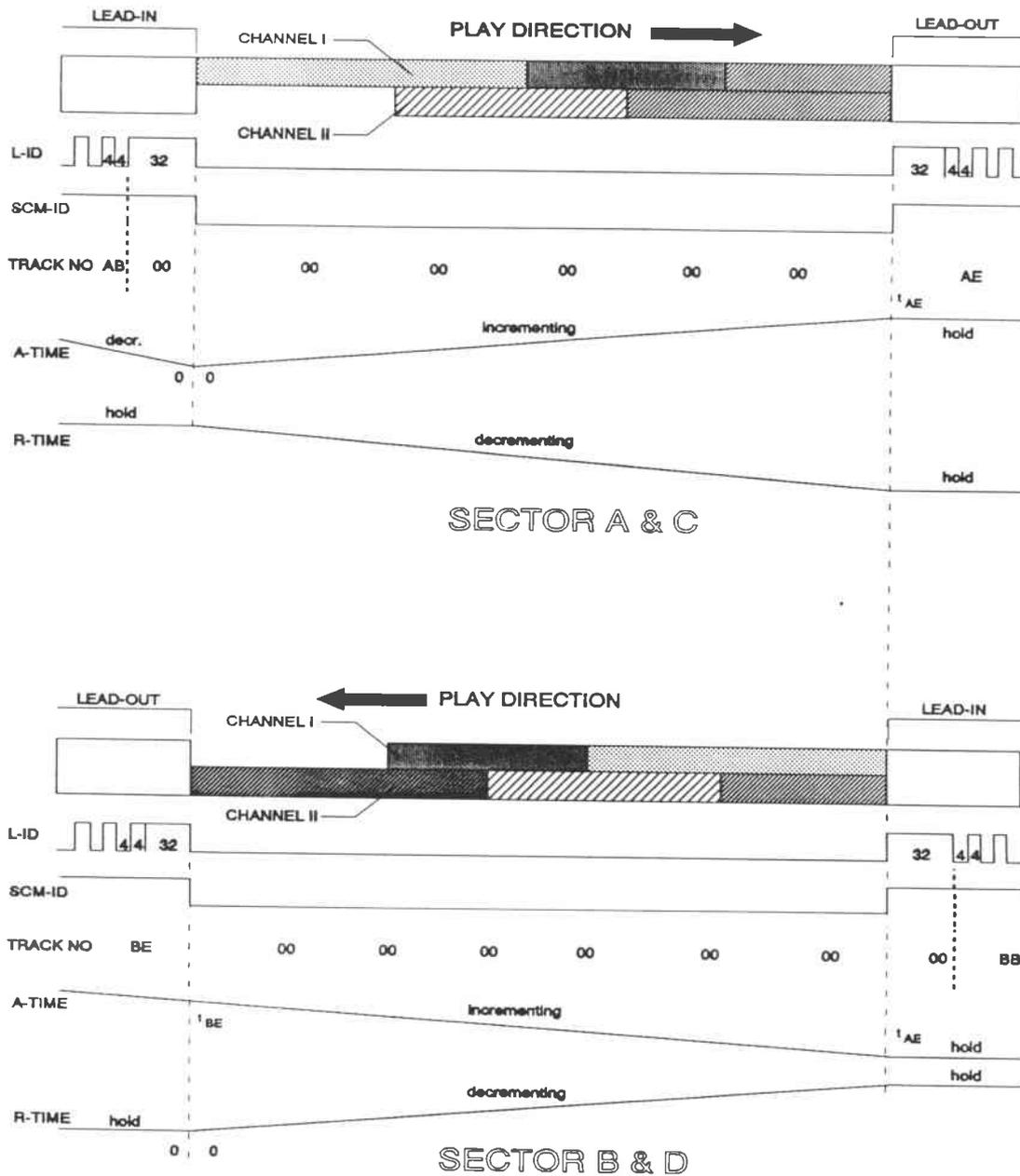
Figure 15.2 : Example of prerecorded 4-Sector tape format
