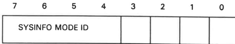
Bits 7-4 are called the Sysinfo Mode ID and indicate the use of the Sysinfo bytes  $SI_5 - SI_{127}$
