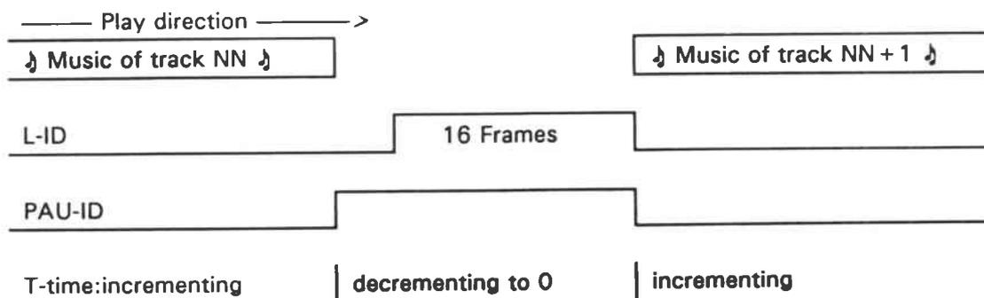
The T-time will increment up to the raising edge of the PAU-ID. Then the T-time will indicate the Pause-time by counting down toward 0:00:00:0 during the pause, and will be 0:00:00:0 at the falling edge of the L-ID, in the last frame just before the start of the music track. The T-time will start at 0:00:00:0 in the first frame of the music track, and will be recorded in ascending order from then on, until the end of the track.
