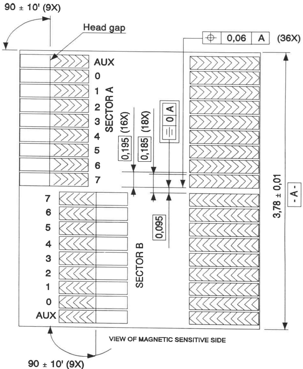
FIG.7.1 : Track configuration, dimensions and identification
