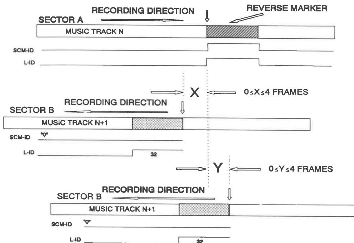
The position of the rising edge of the Reverse marker at the end of Sector A should be 4 frames maximum before or beyond the rising edge of the start marker of the first track on Sector B.
