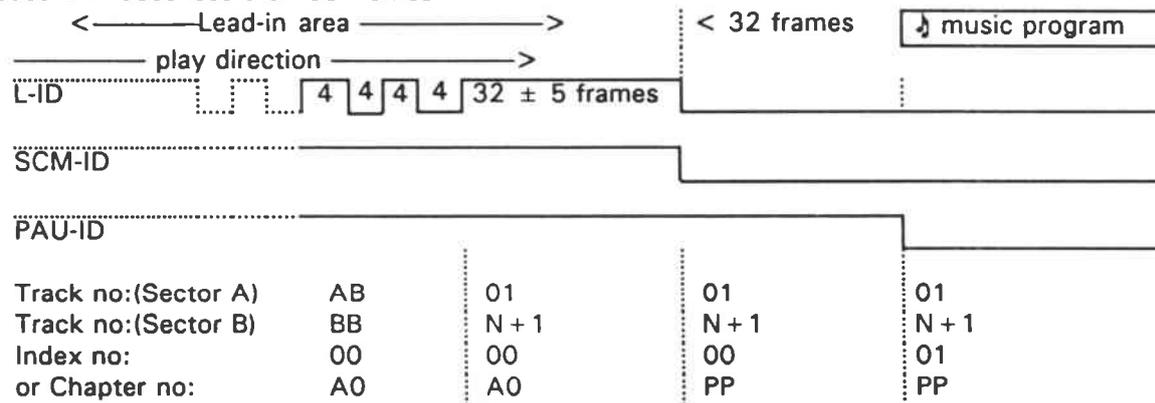
The track number is set at the beginning of the start marker in the Lead-in, the Index number is set to "00" during the pause.
