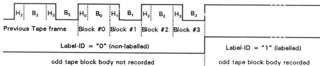
Numbers indicate Tape block numbers in a frame: "H" indicates Header, "B" indicates Body. For the description of the Label ID see chapters 14 and 15.
