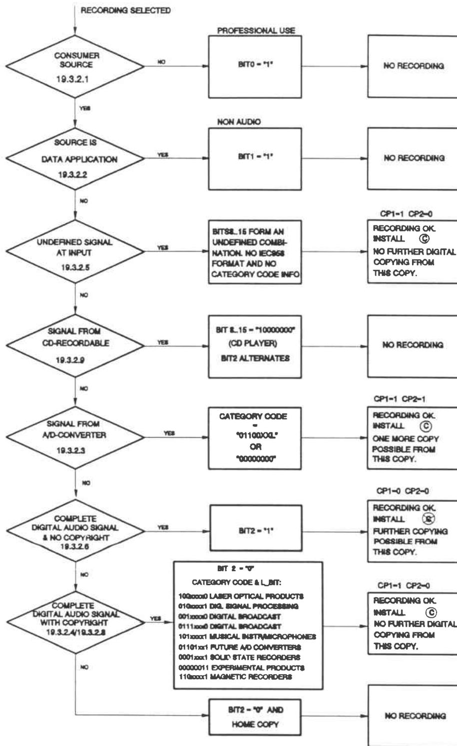
FIG 19.1 SCMS Logic diagram
