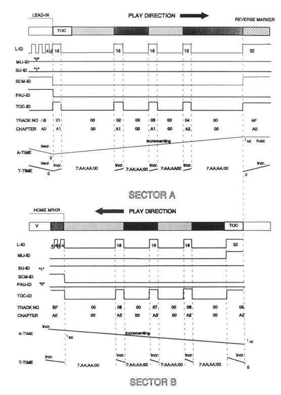
Fig 16.2: Example of consumer recorded super user tape format After renumbering and recording a TOC
