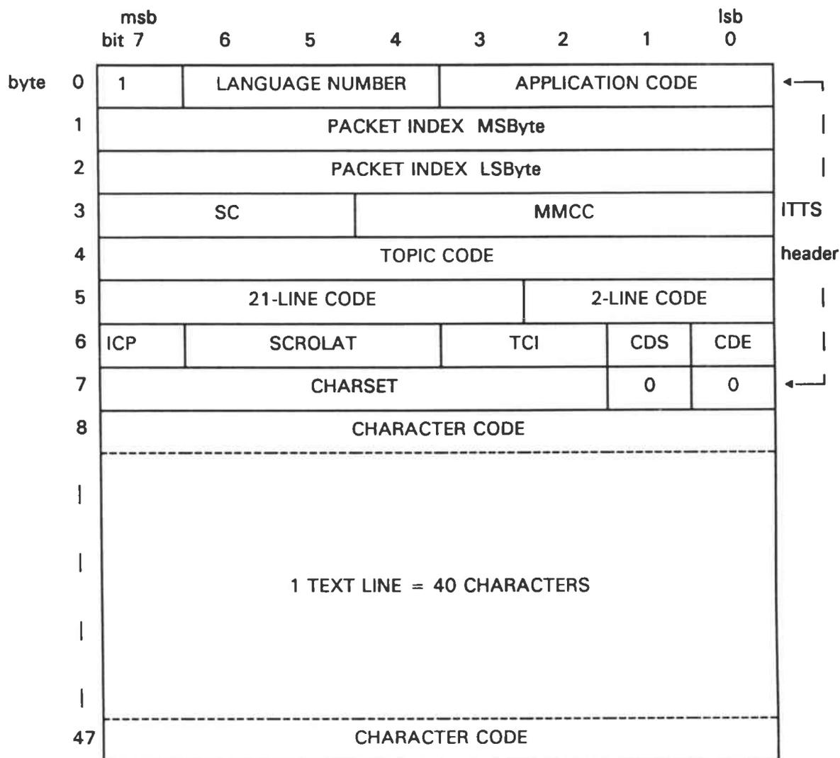
**Note:** The bits indicating a fixed "0" or "1" are reserved for future extensions. Until an application of these bits is defined, the indicated setting must be recorded. In chapter 17 information is given on how a decoder must react if any of these bits is recorded differently.
