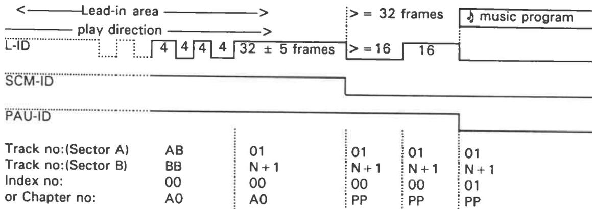
A start marker of 16 frames must be recorded. The track number changes immediately after the Lead-in. Index and Chapter numbers are treated in the same way as in case 2.
