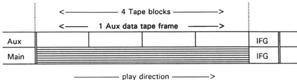
The Aux data tape frames do not have to be aligned to the Main data tape frames. Misalignment may occur in the case of Aux data re-recording, without changing the Main data:
