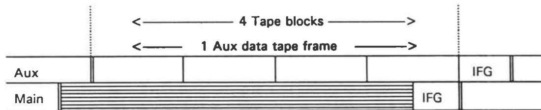
Apart from misalignment, the bit rate of the Aux data can also deviate from 1/8th of the bit rate of the main channel due to variation in the recording tape speed:
