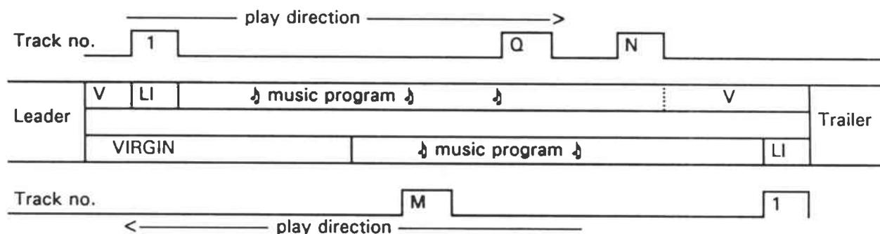
Track numbering shall start at both Sectors with 1. The A-time shall start at either Sector from "0:00:00:0". The SOB bit will be "1" on sector B.
