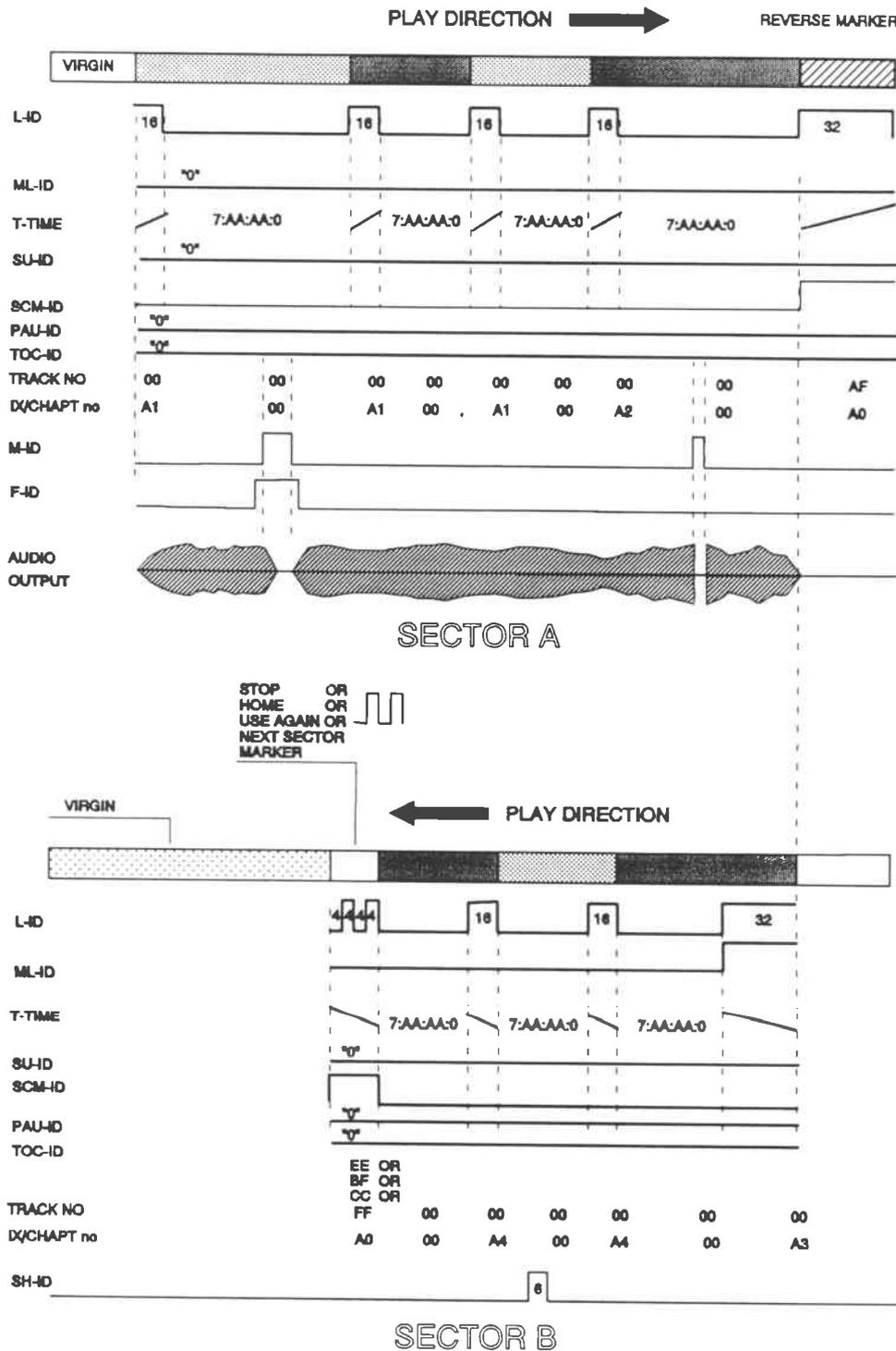
Fig 16.1: Example of consumer recorded user tape format
