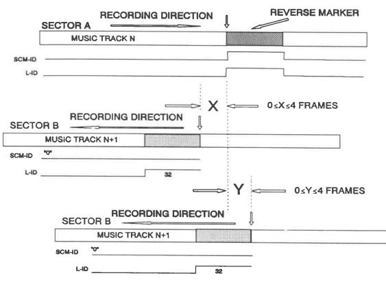
The position of the rising edge of the Reverse marker at the end of Sector A should be 4 frames maximum before or beyond the rising edge of the start marker of the first track on Sector B.
