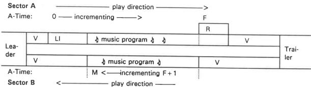
When a Next sector marker has been used (case 2 of 16.2.1), the A-time will start at the Sector B from "0:00:00:0". The SOB-ID is recorded "1". A-time will then be recorded as indicated below:
