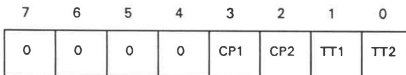
Bits 3 and 2 are called CP1 and CP2 (Copyright Protection bits 1 and 2) and are used to implement the copyright protection system. The following combinations are defined:
