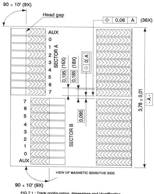
FIG.7.1 : Track configuration, dimensions and identification
