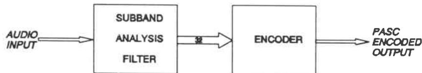
This clause contains a description of the encoding according to the PASC system. Two major blocks are the subband analysis and the transformation of subband data into PASC bitstream.
