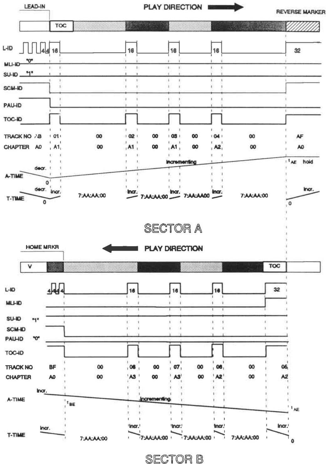
Fig 16.2: Example of consumer recorded super user tape format
