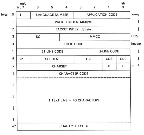
Note: The bits indicating a fixed "0" or "1" are reserved for future extensions. Until an application of these bits is defined, the indicated setting must be recorded. In chapter 17 information is given on how a decoder must react if any of these bits is recorded differently.
