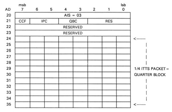
The coding of the Aux data tape block if AIS = 03 is defined:
