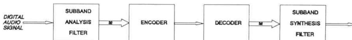
The digital audio input signal is split into 32 subbands. These subband samples are sent to the encoder that determines the accuracy with which the samples need to be transferred. It quantizes the samples according to that accuracy, and adds synchronization and allocation information to form the PASC encoded signal.
