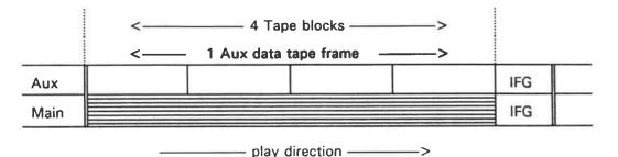
The Aux data tape frames do not have to be aligned to the Main data tape frames. Misalignment may occur in the case of Aux data re-recording, without changing the Main data:
